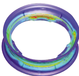
Stresses due to welding and in-service loading
